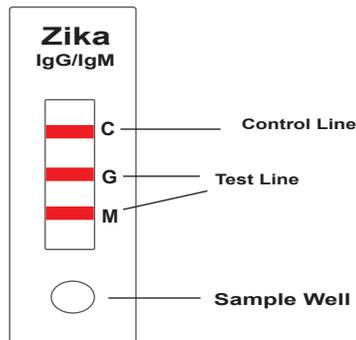
When an adequate volume of test specimen is dispensed into the sample well of the test cassette, the specimen migrates by capillary action across the cassette. Anti-Zika IgM if present in the specimen will bind to the Zika conjugates. The immunocomplex is then captured on the membrane by the pre-coated anti-human IgM antibody, forming a burgundy colored M band, indicating a Zika IgM positive test result.
